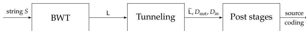
Figure 4.1: Integration of tunneling into the block-sorting compression chain, see also Figure 2.6. Tunneling works as an interim stage. Post stages are, for example, move-to-front transformation and source encoding, see Section 2.2.4.
